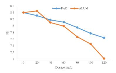
Figure 3: Changes in pH with Dosage 0-120 mg/L
