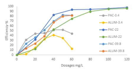
Figure 2: Coagulant Efficiencies 0-120mg/L
