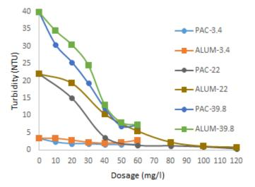
Figure 1: Final Turbidity versus Dosage
