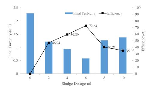
Figure 5: PAC 30 mg/L plus Sludge
