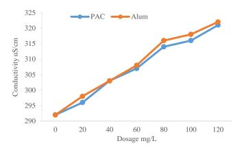
Figure 4: Changes in Conductivity with Dosage, 0-120 mg/L
