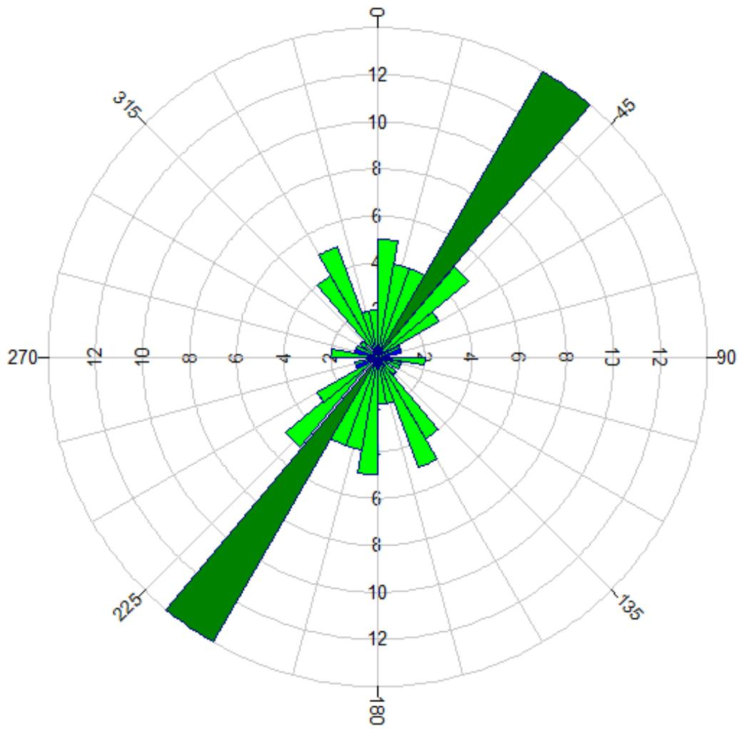
**Fig. 8: Rose Plot of Faults/ Lineaments Features in the Study Area.**
