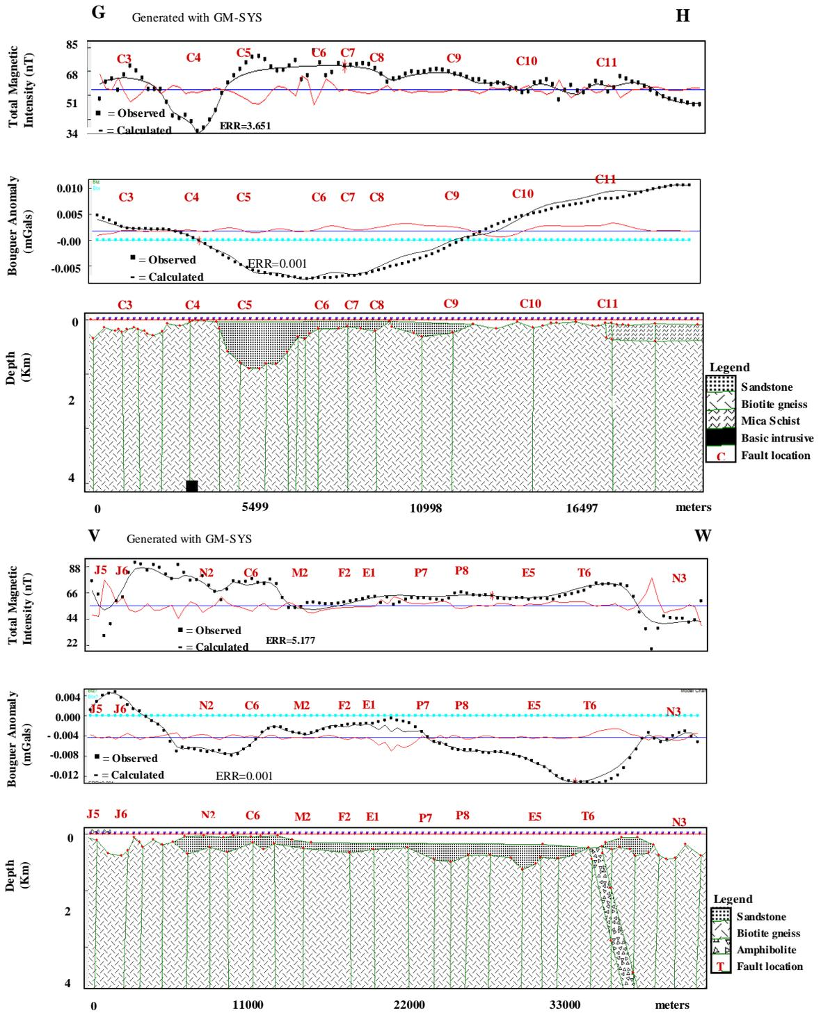
Fig. 6: A Typical Aero-Magnetic, Pseudo-Gravity Anomalies and their Corresponding Earth Model along Profiles GH (top) and VW (bottom).
