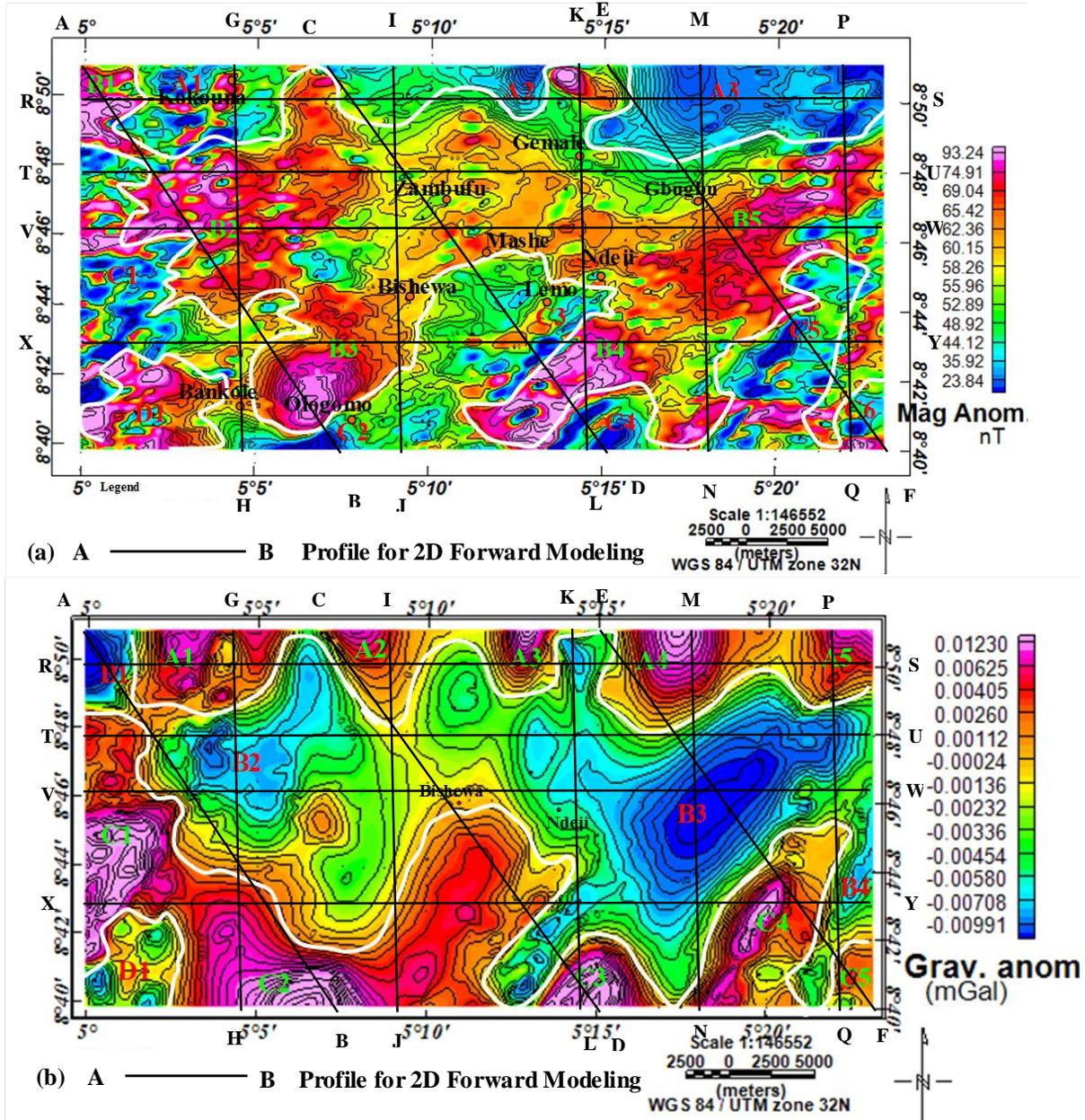
**Fig. 4: (a) Total Field Aeromagnetic Map (REDE) and its Contour**
