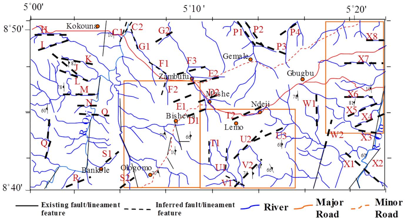
**Fig. 7: Superimposition of Inferred Fault/Lineaments Obtained from 2D Forward Modeling on Drainage Map.**
