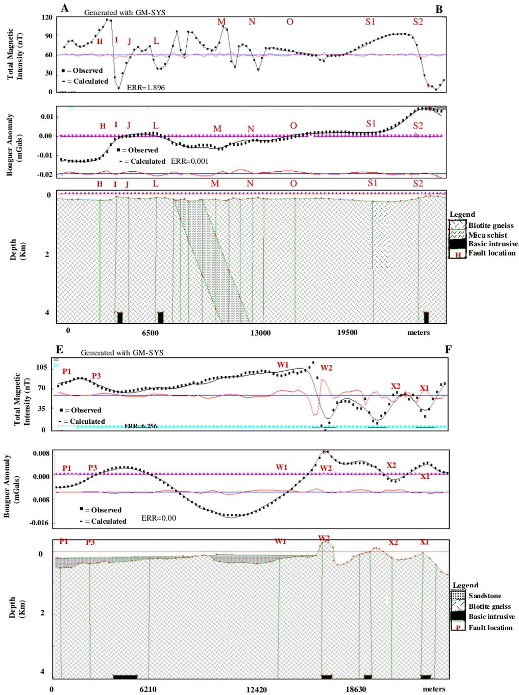
**Fig. 5: A Typical Aero-Magnetic, Pseudo-Gravity Anomalies and their Corresponding Earth Model along Profiles AB (top) and EF (bottom).**
