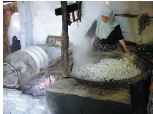
Figure 1B. Silk hand reeling machine
