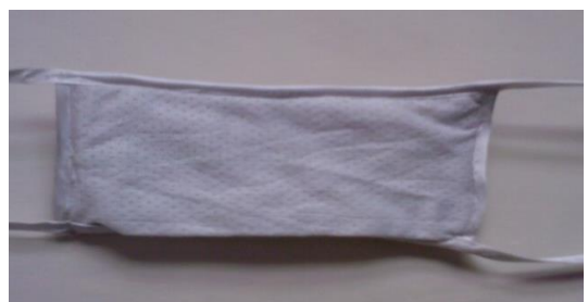
Figure 2: Outer shell bottom side for the proposed affordable and recyclable pad.
