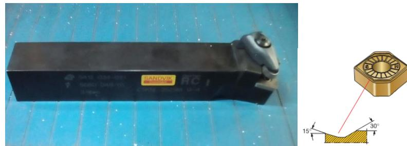
Figure 2: Turning tool holder and cutting tip used
