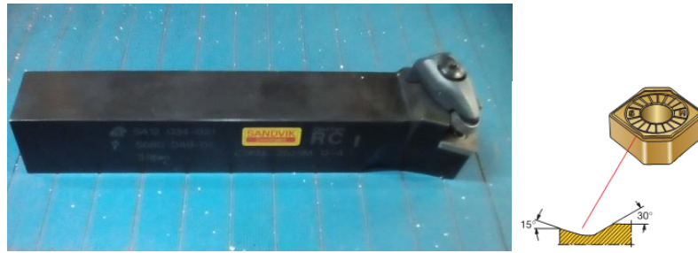
Figure 2: Turning tool holder and cutting tip used
