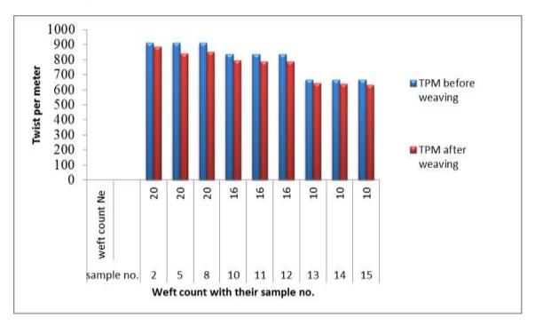
Figure 1. Twist of different weft count before and after weaving
