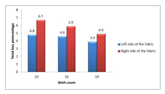
Figure 3. Twist loss at the left and right side of different samples
