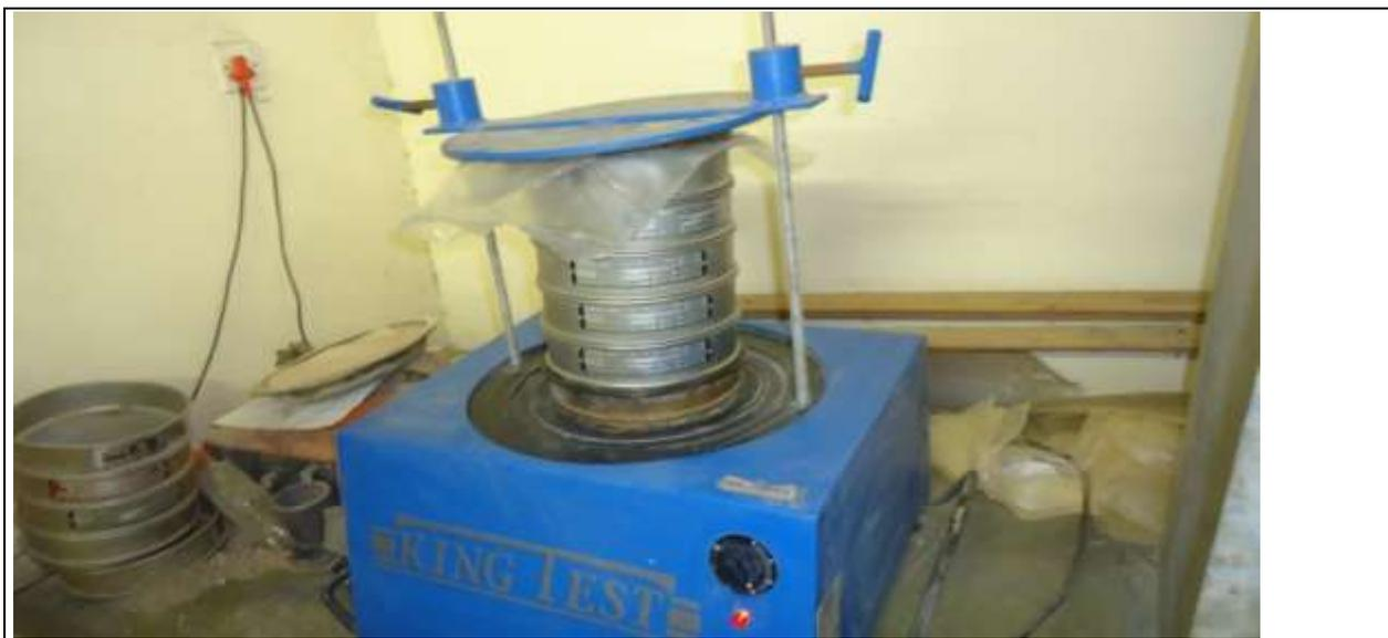
**Fig 1. Sieve shaker (ZSM Department of Metallurgy Laboratory)**
